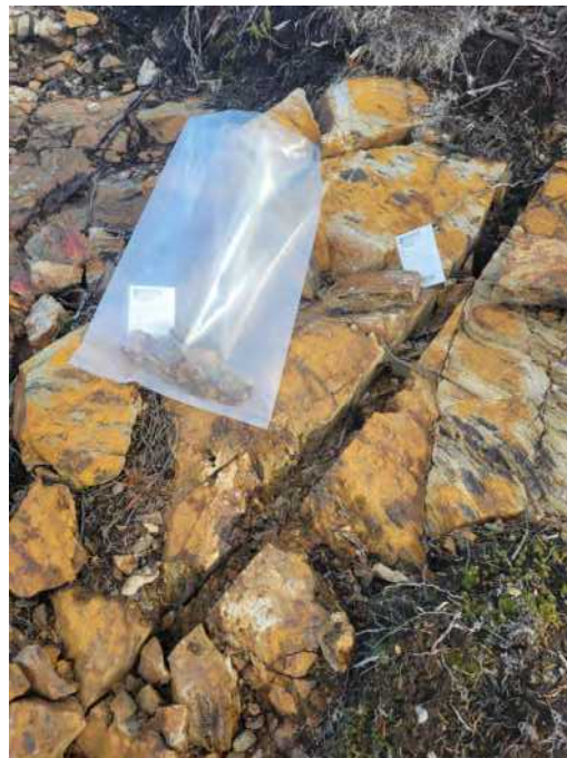
Figure 23. Re-sampling of disseminated pyrite in felsic volcanic rock with quartz veining in previous sample channels at the TD500 showing returned 696 and 871 ppb Au.
