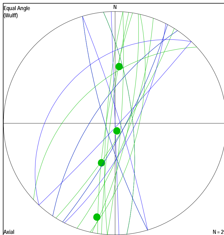
Figure 7: Stereonet of Structural Measurements Collected in the Thurber Dog Area. Foliation as Green Great Circles, Veins as Blue Great Circles, Mineral Stretching Lineations (Along Foliation) as Green Poles.
