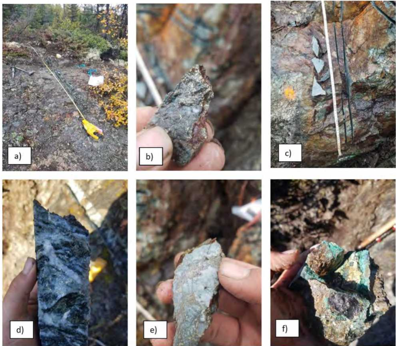
Figure 37. Kaapak copper showing. a) Channel cut across quartz vein hosting chalcopyrite mineralization. b) Chalcopyrite mineralization in host rock. c) Channel cut through chalcopyrite rich zone d) Brecciated host rock with quartz vein, peppered with chalcopyrite. e) Semi-massive chalcopyrite from channel sample. f) Weathered mineralized zone with strong malachite.
